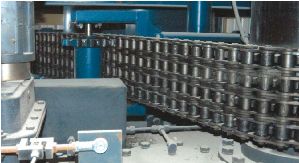
FALK column rotation drive with sprocket, chain and load cell
